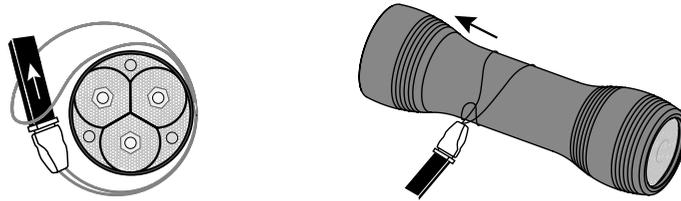
**WARNING:** If looping around a handlebar be sure to do so enough times that the light cannot fall into the front wheel.
