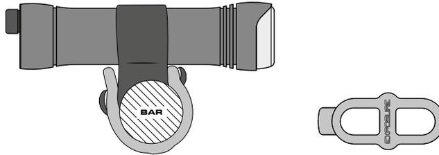
The shorter arm of the **QR Handlebar Mount** bracket faces the front. The tab-end of the silicone band fastens on the rear.
